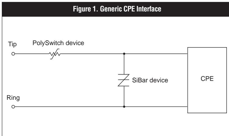
PolySwitch devices should be selected with voltage ratings based on the regulatory standards for which the equipment is being designed. Surface-mount TS600 or TSM600 and radial-leaded TR600 devices are applicable for North American GR-1089 standards and for UL60950 standards, while surface-mount TS250 and TSV250 and radial-leaded TR250 products are applicable for ITU-T K.21 standards.
