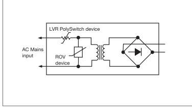
Figure 1. Transformer Circuit
