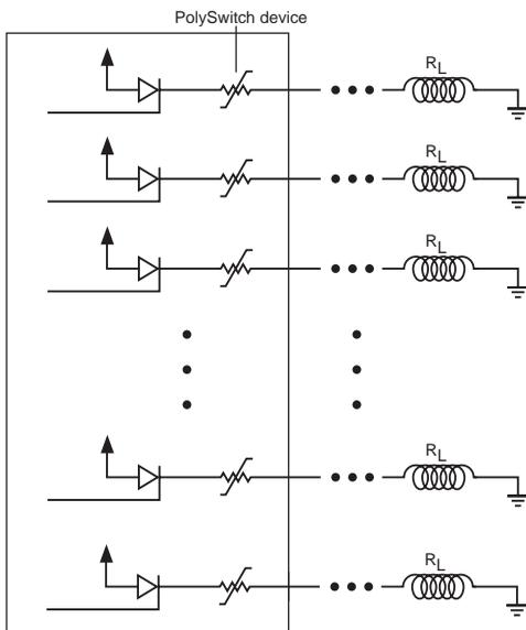
A protection scheme is also noted in Figure 4. Since these sensor lines can cover long distances, they are typically found in the same conduit with other voltages. If an overvoltage situation should occur, and the rail voltage of the op-amp is exceeded, the overvoltage device will immediately break down. The PolySwitch device will then trip if the fault is prolonged, helping to protect the circuitry, including the overvoltage device.
