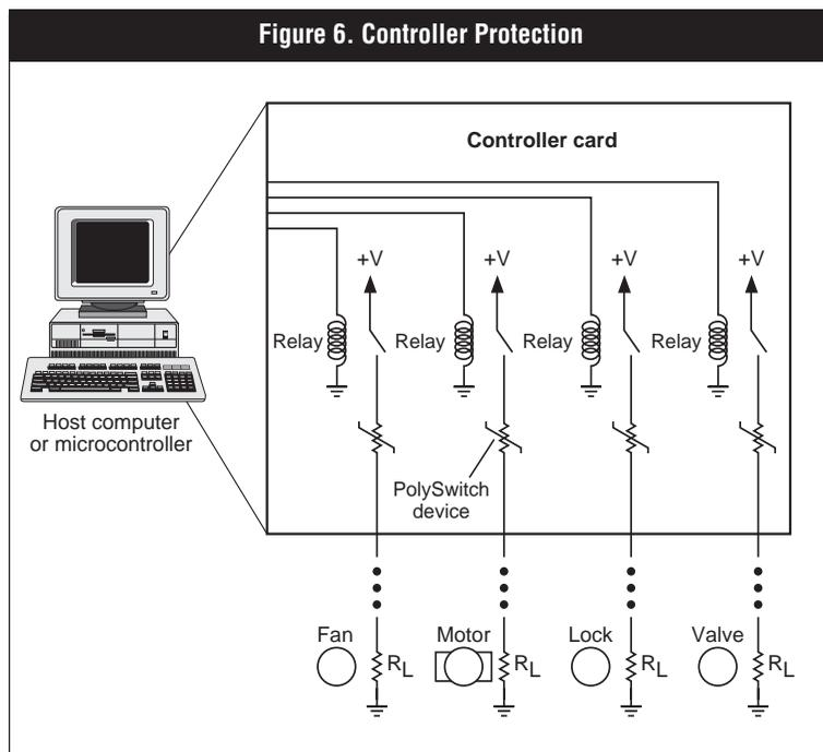
A long-standing tradition that contributes to miswiring is that both power (less than 100 V<sub>DC</sub>) and signal lines are often run in the same conduit. At the remote end, which can be thousands of feet away from the host, it is not difficult to connect the wires incorrectly, wire the hot lines to ground, or superimpose powered lines on low-voltage data lines.
