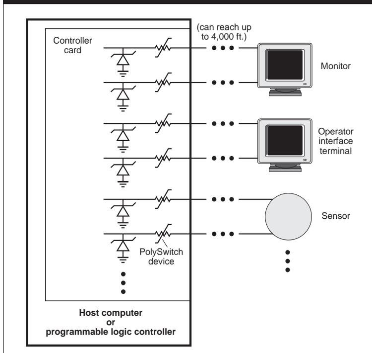
**Figure 3. Data Acquisition Architecture**
