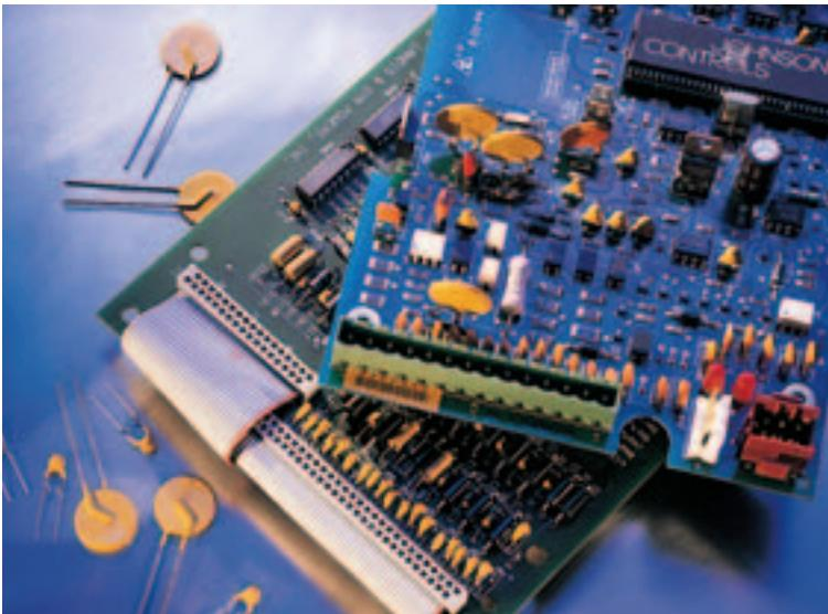
device such as an RXE010 device. Circuit protection would be placed immediately after the interface to the printed circuit board before the transceiver for the twisted pair.
