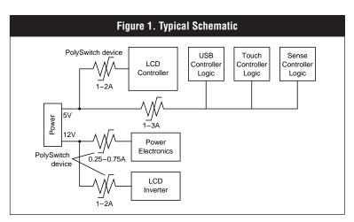
Raychem Circuit Protection LCD Monitor Controller/Inverter 119
